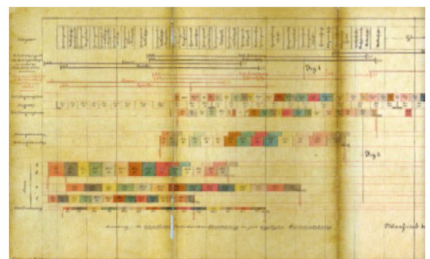
Fig. 8: Graphical depiction of the progress of work on the Gotthard Tunnel in 1876
